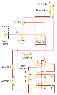
A counter-EMF opposes any change in current flow and is used to reduce high-starting currents.
