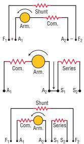
NOTE: Standard rotation for <u>DC generator</u> is clockwise.
